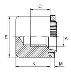
Female thread A = M6Height K = 11.0Min thread length C = 6.0Outer diameter E = 13.0Plate thickness = 3.5 to 3.7
